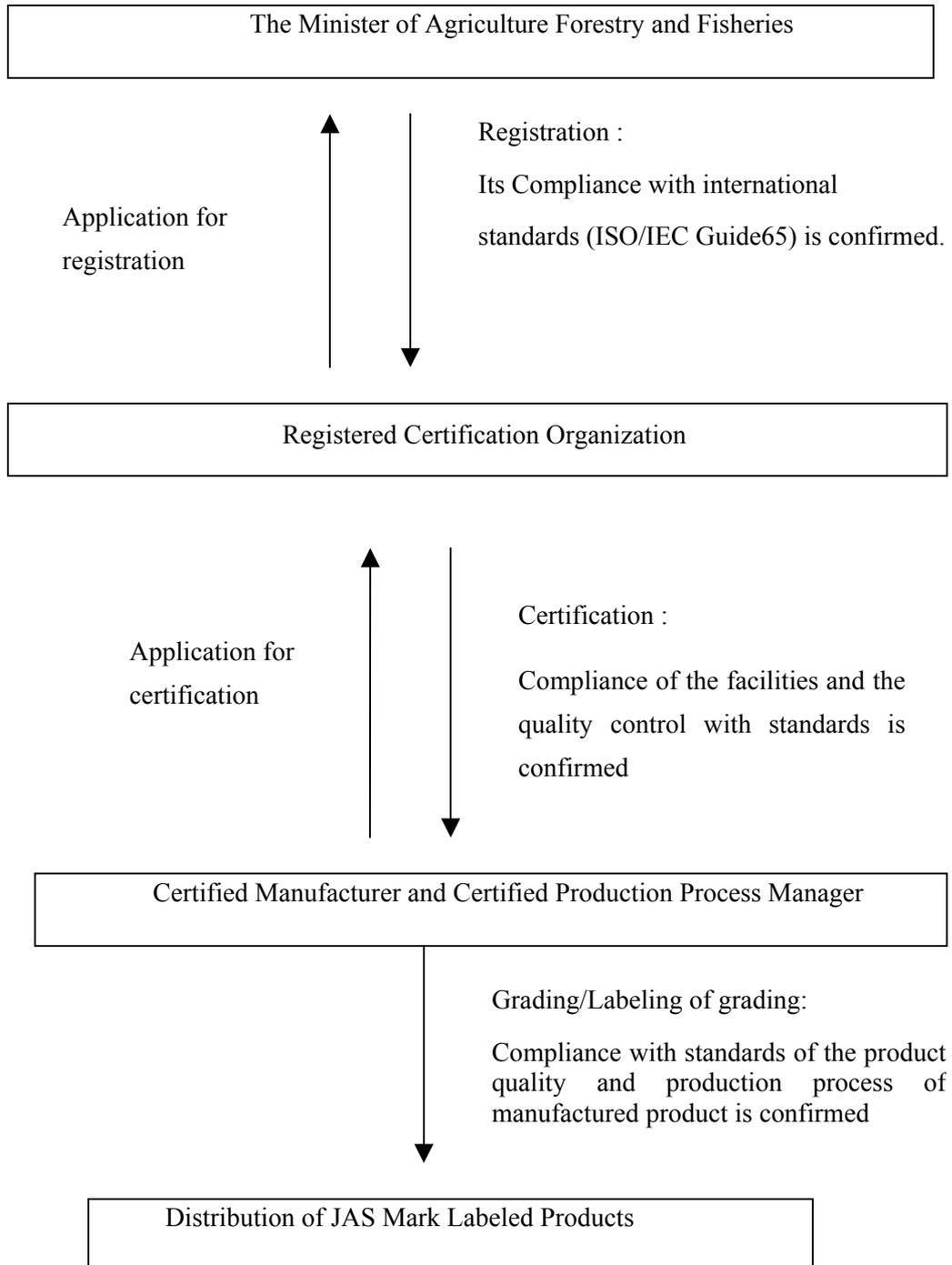
(b) Inspection method for the grading
